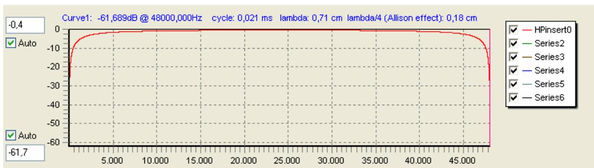
For better understanding of the mirror effect the previous picture in addition shows the frequency response of the corresponding highpass filter (Linkwitz-Riley 1<sup>st</sup> order 1 kHz) after zero insertion.
