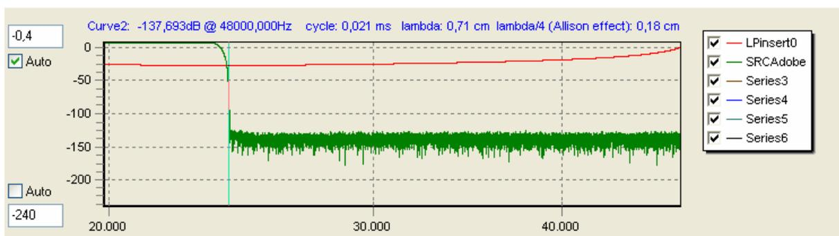
As the filter is given in 32 bit single float precision the noise level is higher, the noise floor is at about -130 dB.
