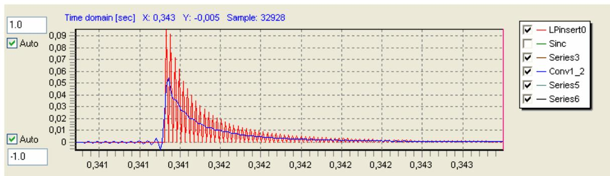
The blue curve has lost the big jaggging at the first sight. We also notice a lower amplitude of the time domain signal whereas in the previous picture the frequency response of the filtered signal has the same amplitude as the original signal, but only below 24 kHz. Indeed we have to apply a gain of factor 2 to compensate for the energy loss and to get the same signal height in the time domain.
