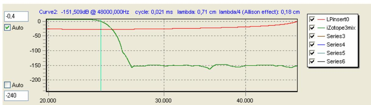
The falling slope in the transition area looks a bit disturbed whereas the stop band looks pretty nice.
