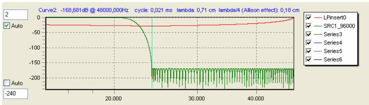
The filter transition area stops at 24 kHz. The stopband shows the equiripple design underlying the filter design.
