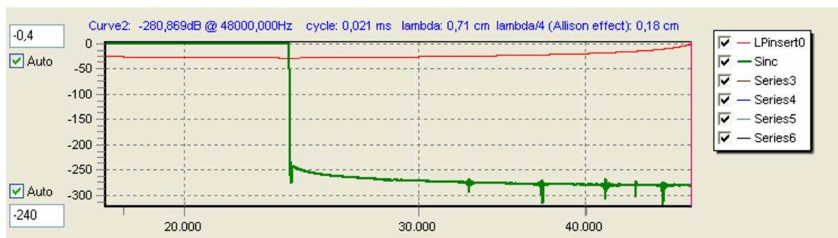
The zoom-in shows this a bit better. All frequencies above 24 kHz have a much lower level, here below -250 dB. The theoretical sinc filter is endless deep. But we must taken into consideration that the number resolution is 64 bit double float and the length of the sinc filter is 65536 samples. A perfect sinc filter indeed would have infinite samples.
