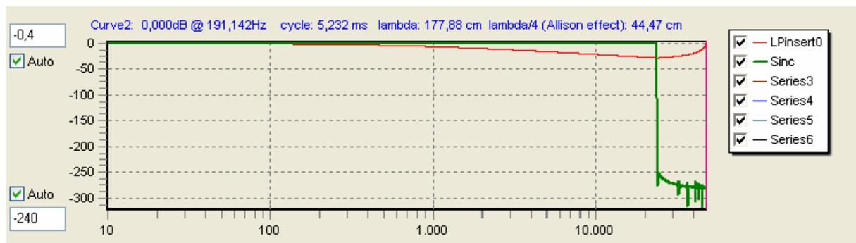
The 24 kHz sinc filter shown as green curve has a steep cut of all frequencies above 24 kHz.
