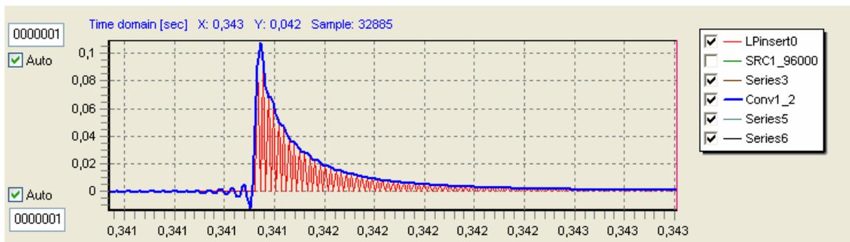
The result is the smoothest result of all. But in the given case we also need to keep in mind that the filter is given in 64 bit resolution whereas the Adobe Audition and iZotope RX Advanced filters are given in 32 bit resolution.
