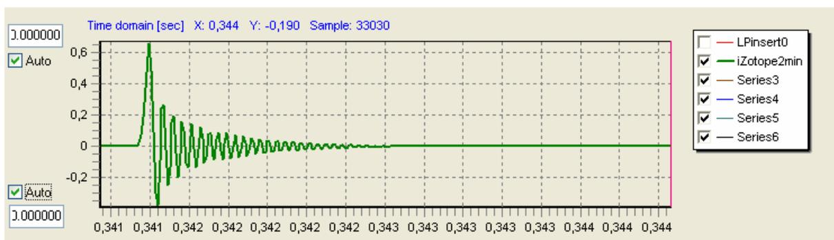
This is clearly a minphase filter. The filter length is also 266 samples.
