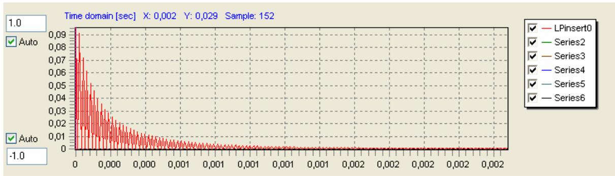
So with the same timescale in the bottom axis the signal looks compressed. We have double samples in the same time.
