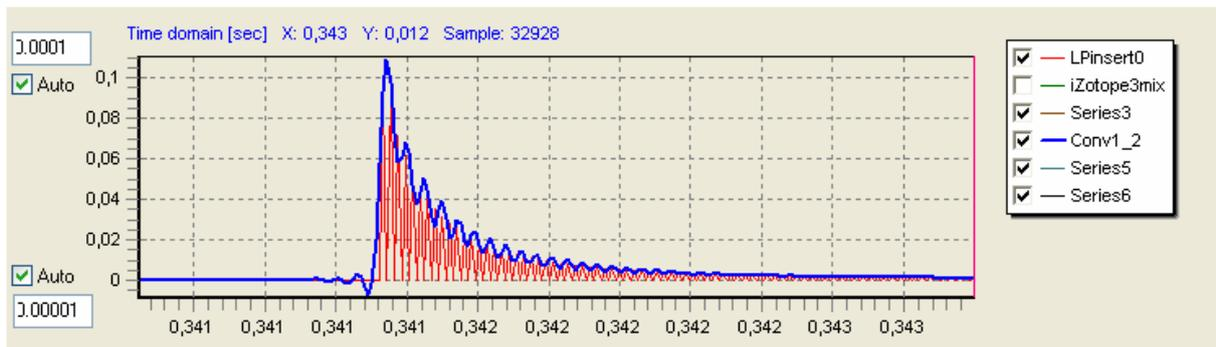
Now the delay of the pure minimumphase filter has gone. The filtered signal looks a bit more smooth too. But the quality of the shape of the linearphase filter is not met. As already said the mixed phase filter is a compromise.
