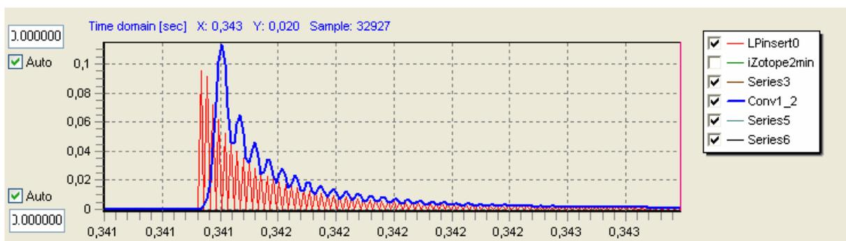
Beside the small introduced delay it can be clearly noticed that the minimum phase filter does not smooth as well as the linear phase filter.
