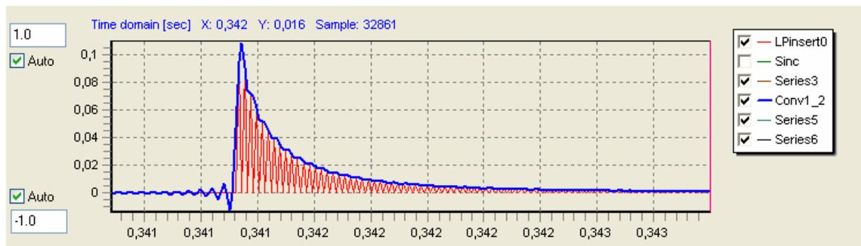
The convolution with the sinc filter has also introduced a time delay of  $32768/96000 = 0.341333..$  seconds. For better comparison the signal with zero insertion is shifted accordingly by the same amount of delay.
