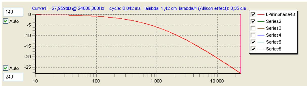
Frequency response of the lowpass filter. Max. frequency is 24 kHz according to Nyquist
