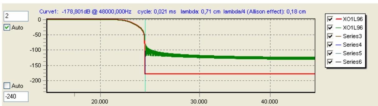
And to show how this filter with 1500 taps compares against the iZotope filter with 266 taps:
