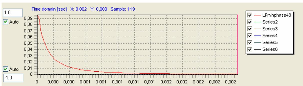
Pulse response of the lowpass filter. Shown are the first 120 samples of the minimum phase filter.
