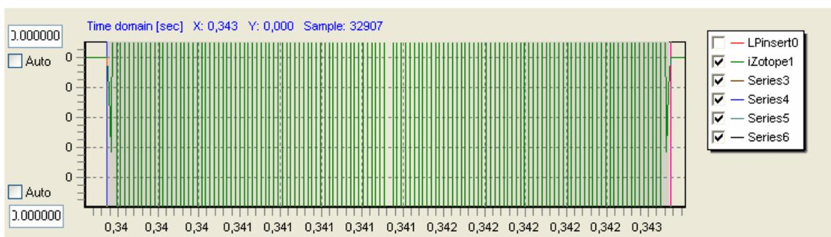
Filter length is 266 samples. A very short filter of roughly 2.8 ms duration, 1.4 ms pre-ringing.
