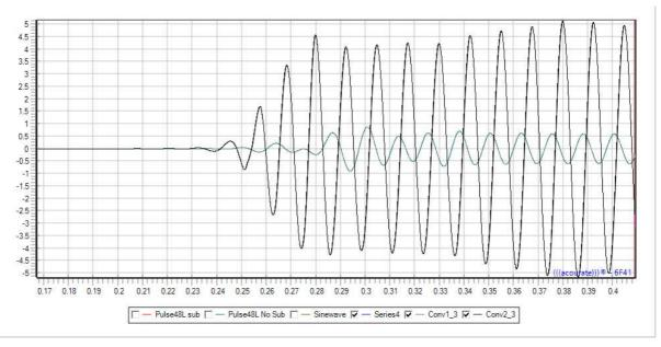
Well, we clearly recognize a pretty low signal amplitude of the subwoofer in comparison to the main speaker. A first approach would be to adjust the gain of the subwoofer in relation to the main speaker, if possible. We can even adjust this by applying some gain to the measurements.
