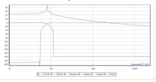
The picture shows the frequency response of a lowpass and a highpass crossover NT2 with a corner frequency is 80 Hz. Furthermore the picture shows an 80 Hz sinewave created by Generate – Sinewave – 80 Hz
