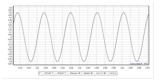
Indeed in the perfect world both convolution results match in phase (because of the linear phase filters) and amplitude (0.5 = -6 dB point @ 80 Hz). So in the steady state we expect the results to be in phase, otherwise we do not match the timing requirements.
