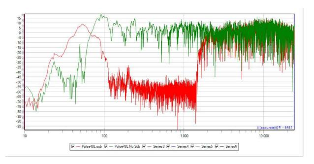
The picture shows two frequency responses. The green one is the main speaker without subwoofer. The red one is the subwoofer plus the main speaker treated by a highpass. This allows the pulse responses to be perfectly time aligned by the high frequency content in the responses. Because the high frequency content creates a peak with a high amplitude.
