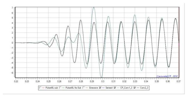
So in the steady state sub and main speakers are running together. But at the very first start we do not get the transition that we like to have.
