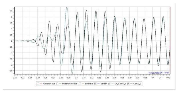
The picture shows the result with the sub polarity switched again and playing the sub 277 earlier than the main speaker.
