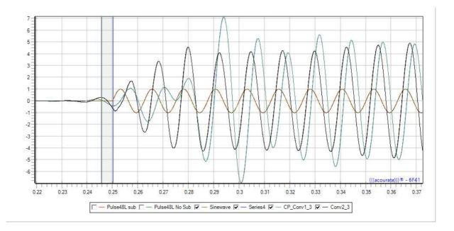
The left marker shows the positive peak of the main speakers left transition, the right marker shows the negative peak of the sub. We expect the left transition zone to be in opposite.
