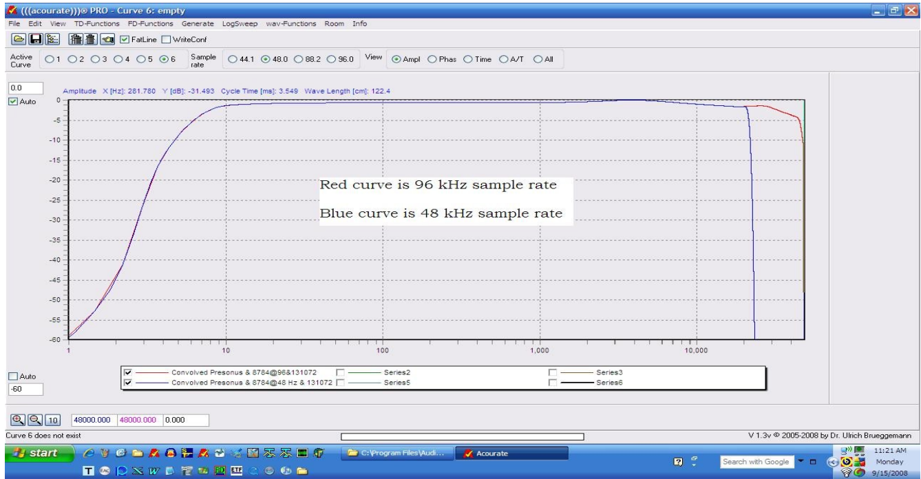
Figure 2. Convolved calibration for Presonus Firebox and Earthworks QTC 50 Microphone
